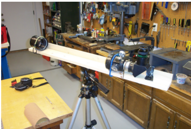
Paul Lind's "Focal Length Measuring Tool" with the 3" lens and focuser
