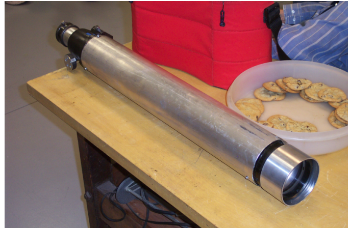
The 3" Refractor telescope assembled into a 4 inch tube
