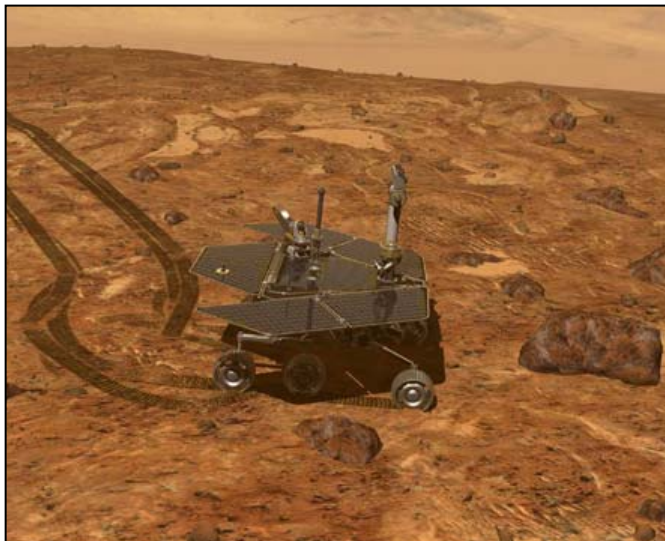
Opportunity spots a rock with its NavCam that its AEGIS software says meets all the criteria for further investigation.
