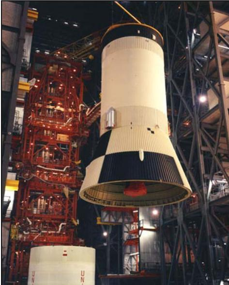
*The S-IVB 3rd stage being lowered to the S-II 2nd Stage. The conical adapter would separate with the S-II. The big silver lump on the side at the top of the adaptor is one of the ullage Motors*
