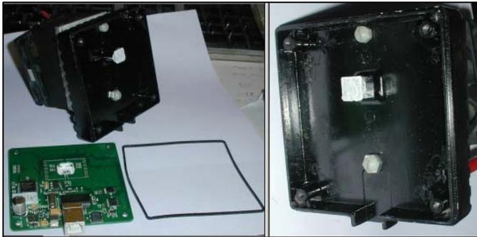
Figure 4-Inside the DSI Pro with Cold Finger shown
