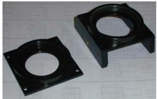
Figure 3-Low Profile Adapter (left) and Original
