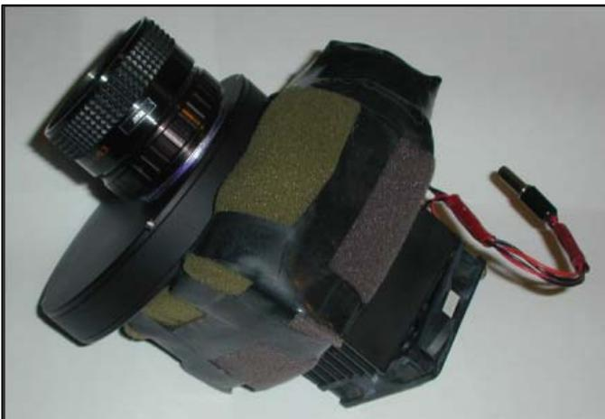
**Figure 7-Modified DSI Pro with Foam Insulation**
