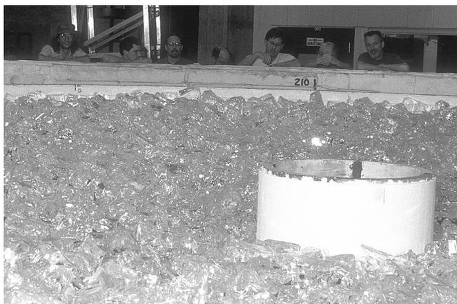
Photo by Dean Ketelsen. The mould was filled with 11 tons of glass. Each piece is roughly brick-like, in size, shape, and weight.
