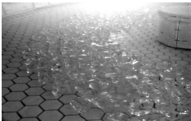
Photo from the Steward Observatory Mirror Lab Web Page. Two tons of new glass has been added and the mirror is being reheated once again.
