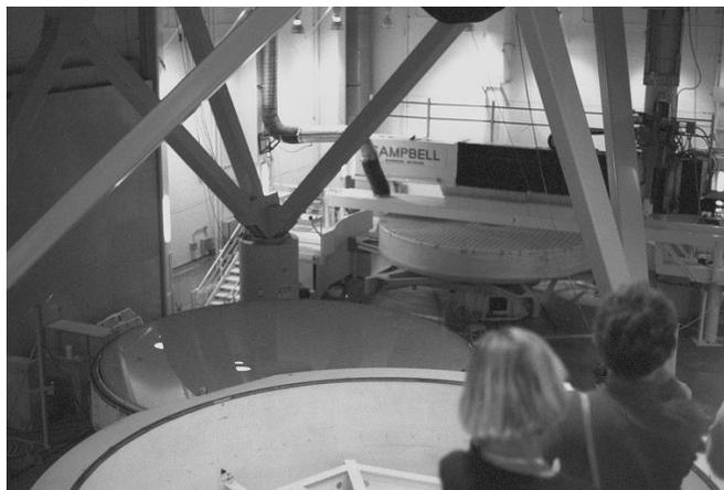
Photo by Paul Dickson. In the foreground is the mirror cell for holding the new MMT 6.5m mirror, which lies just above it in the photo. The second 6.5m mirror lies face-down on the grinding platform just above the first mirror. The back of the mirrors are ground to relieve stresses in the glass.
